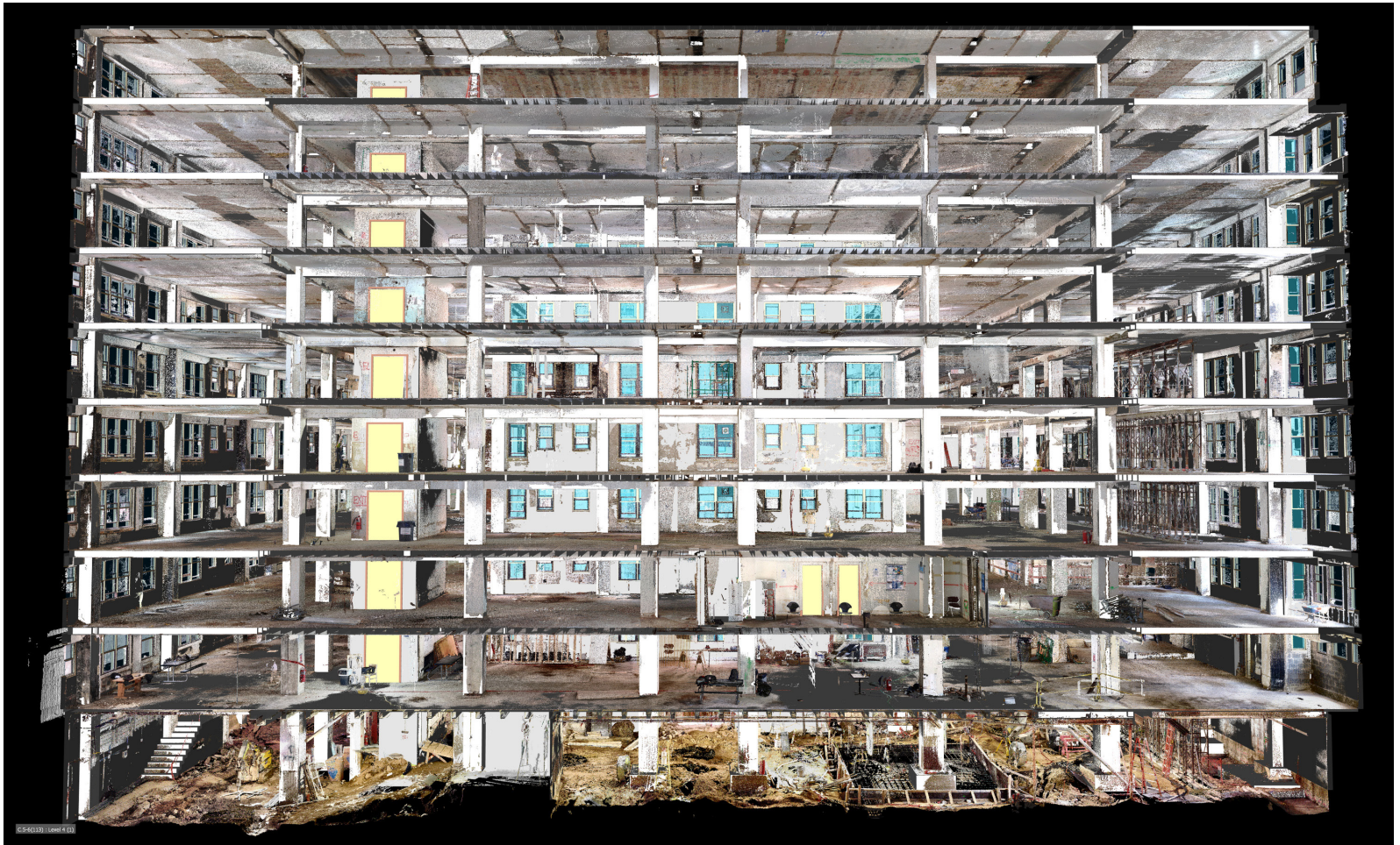
The Coda team developed 3D models of the existing structure with 350 scans and 648 precisely modeled individual concrete beams.
