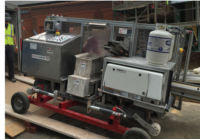
SAM100 arrives at the Lab School of Washington jobsite (above). Bricks are picked up by SAM's robotic arm, mortared, and placed on the wall (left).
